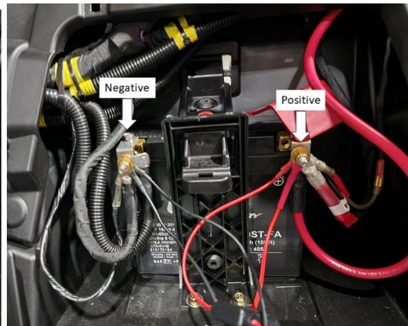
Remove the battery cover by pulling outward from the top. Using a 10mm wrench, remove the negative battery cable followed by the positive.
