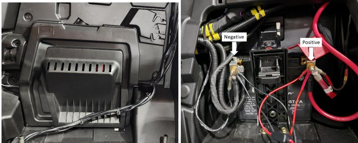
Using a 10mm wrench, reinstall the positive battery cable followed by the negative. Reinstall the battery cover by engaging the top two clips. Test light functionality.
