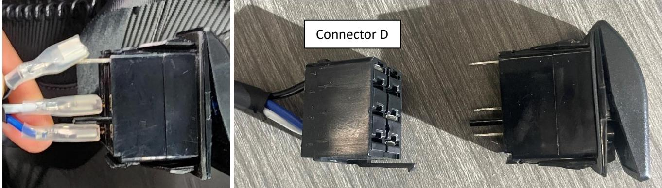
Remove the Rocker Switch(s) from Harness and **NOTE THE POSITION OF EACH COLOR CABLE.**
