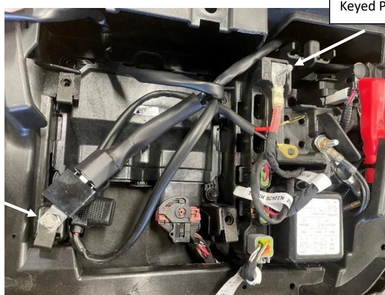
**Step 16: Route harness as shown. DO NOT attach connector onto exposed wire harness pins.**
